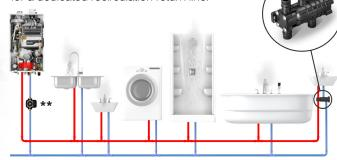
PFFW-SXX-001, NaviCirc Kit: 30022965A. \*\*External recirc pump and check valves not included.
